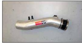
24. Install the two  $\frac{1}{4}$  NPT crankcase vent fittings into the K&N® intake tube as shown.
