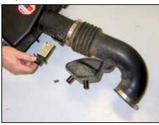
19. Remove the mass air sensor from the stock intake tube as shown.
