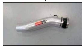
21. Install the provided silicone hose (08051) onto the K&N® intake tube as shown and secure with the provided hose clamp.
