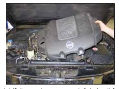
4. Lift the engine cover and dislodge it from the mounting grommets and then remove the engine cover from the engine.
