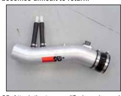
25. Attach the two modified crankcase hoses onto the  $1\!\!/\!_{\!4}$  NPT fittings.
