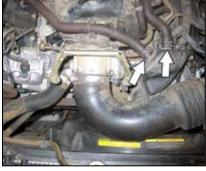
5. Release the two spring clamps which secure the crankcase vent hoses to the intake tube and then disconnect the crankcase vent hoses from the intake tube.
