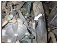
16. Remove the engine ground strap mounting bolt shown.
