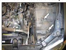
9. Remove the two airbox mounting studs shown from the inner fender.
