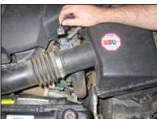
2. Disconnect the mass air sensor electrical connection and unclip the wiring harness from the airbox.
