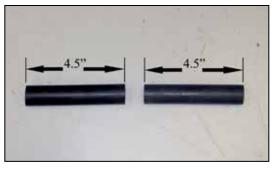
22. Cut the provided crankcase vent hose into two 4.5" sections as shown.
