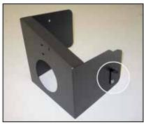
10. Install the heat shield mounting bracket (07805) onto the heat shield as shown using the provided hardware.
