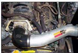
26. Install the K&N® intake tube assembly and secure to the mounting bracket and silicone hose with the provided hardware and hose clamp. Then connect the crankcase vent hoses to the factory hoses as shown.
